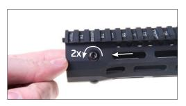
**3.** Loosen the four screws by two full turns with 5/32 allen wrench. (provided)
