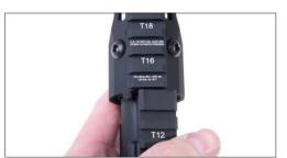
4. Slide rail onto barrel nut while rotating rail 5 degrees "clockwise" until flush with receiver, then rotate back to align rail with upper receiver.
