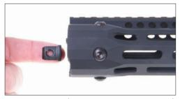
2. Install the clamps (tappered end towards the barrel nut) and screws provided and tighten until they're snug.
