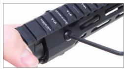
**5.** Holding rail into position, tighten the four retaining clamp screws evenly. (For best results use thread locking compound.)
