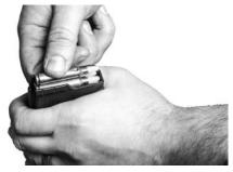
Always place bullets into the magazine from the top. Place bullets down onto the follower and depress until the feed lip holds the bullets. Continue to load until the desired amount of bullets is placed into the magazine.
