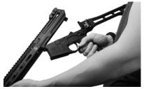
To remove front take down pin, rotate pin clockwise and remove to separate Upper and Lower Receiver
