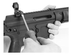
Place the sight base and sight base clamp onto the rail and hold tightly together. While still clasping, use a drop of thread locking compound while you tighten the screw to fasten the sight to your rifle. (Note: Sight should fold to rear of rifle).
